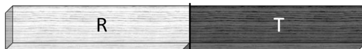
Figure 10: Material allocation for references (R) and thermal modification (T) from one board
