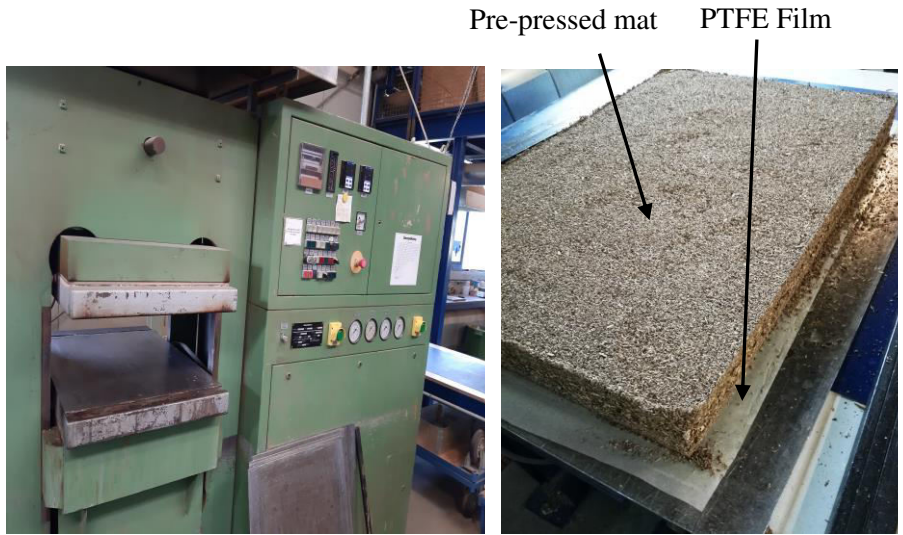
Figure 26: Hot press from the company Siempelkamp, D-47803 Krefeld (Left), and pre-pressed mat ready for hot-pressing (Right).
