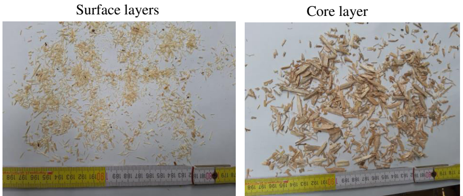
Figure 14: Laboratory produced core layer and surface layers wood chips. The ruler at the bottom is marked in cm.
