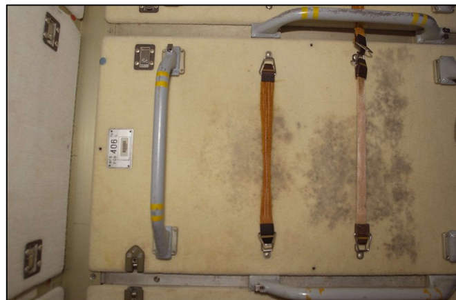
Figure 1: Fungal biofilm contamination aboard the ISS
