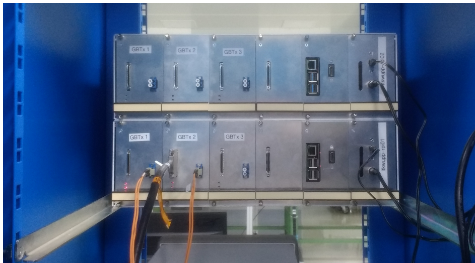
Figure 5.11.: Picture of the readout rack next to the demonstrator with both readout boxes installed.
