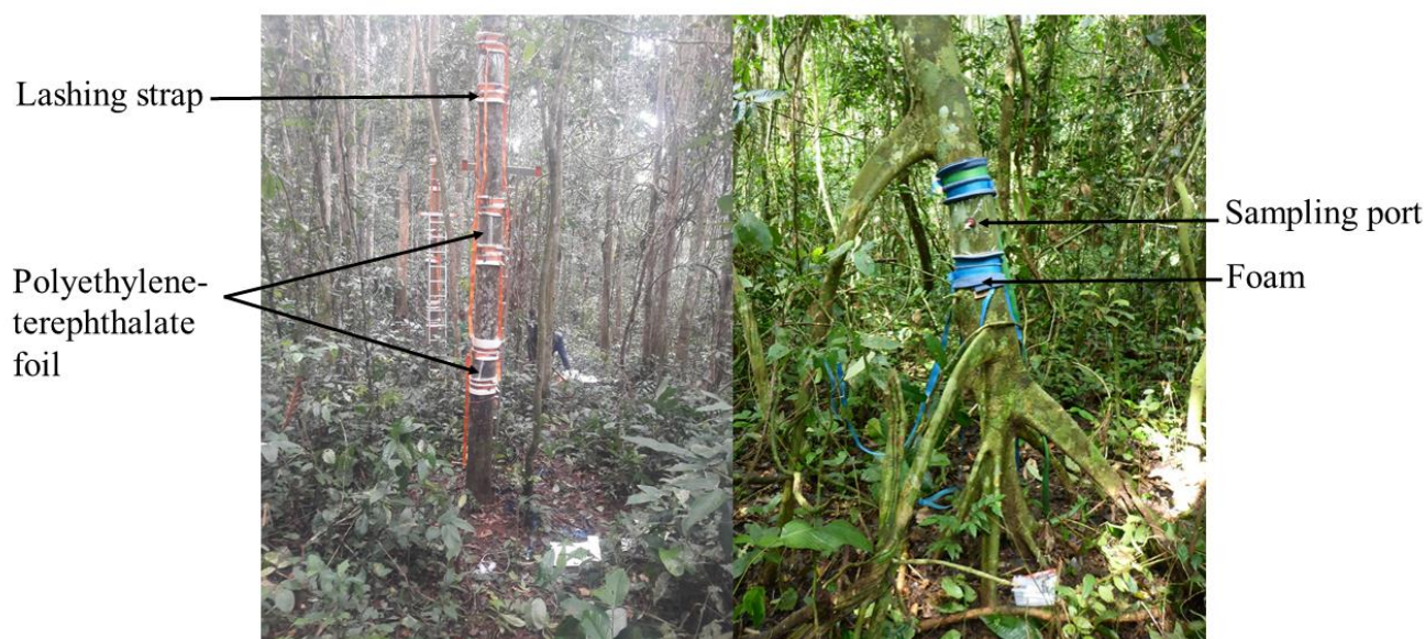
Figure 2.2. Sampling set-up for stem nitrous oxide ( \text{N}_2\text{O} )-flux measurement at three stem heights in a rainforest in the Congo Basin, Cameroon.
