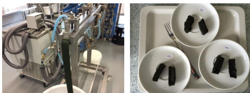
Figure 5.1: To the left, the extruder is shown, while one of the spirulina-soy extrudates is produced. This “endless” string of sample was cut into blocks of 300 g from which the strips of 10 g (right picture) were cut prior to cooking for sensory evaluation.
