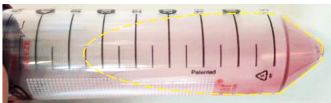
Figure 5.11: Film-like of silica-planet-gold-satellite nanostructures collected by the centrifugation process (6000 rpm, 20 min) with the aid of additional water in the colloid. Yellow lines highlight the area of collected nanoassemblies.
