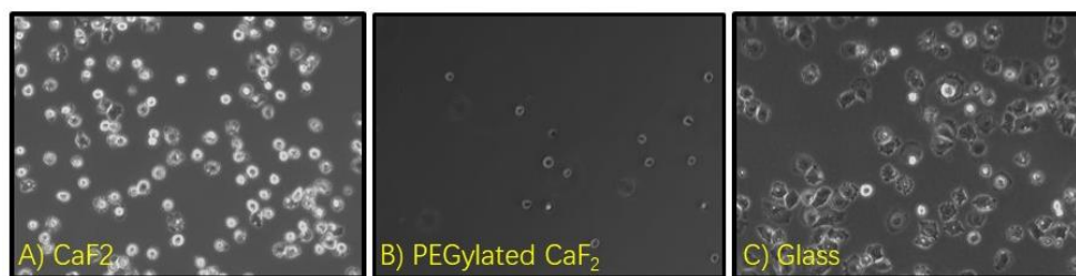
Figure 5.16: Micrograph of remaining melanoma cells on the substrate after incubation and rinsing with water. A) Plasma treated \text{CaF}_2 surface. A significant amount of cells are attached to the surface while maintaining its spherical shape. B) PEGylated \text{CaF}_2 surface. The number of attached cells is significantly reduced compared with A). C) Plasma treated glass surface without passivation. Cell spreading can be observed here indicating a strong interaction between unprotected glass surfaces and cells.
