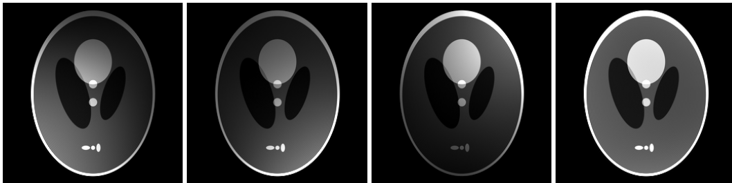
Figure 2.1: Illustration of parallel imaging: Three simulated channels of a Shepp-Logan phantom (radially sampled) and root sum squares composition from a total of eight channels.
