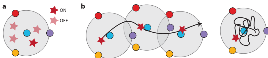
Figure 1.2: Experimental modalities of MINFLUX. a , MINFLUX imaging using an on-/off transition to acquire single molecules (red stars) sequentially in time [6]. Colored dots represent the TCP. b , MINFLUX tracking to follow single, continuously emitting molecules (red stars) over extended regions (left) [6] or within the confined MINFLUX FOV (right) [26].
