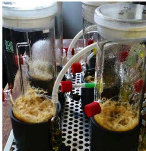
Figure 6. Hairy root cultures generated from several accessions of Hyoscyamus niger in bioreactors operated in a bubble aeration mode.
