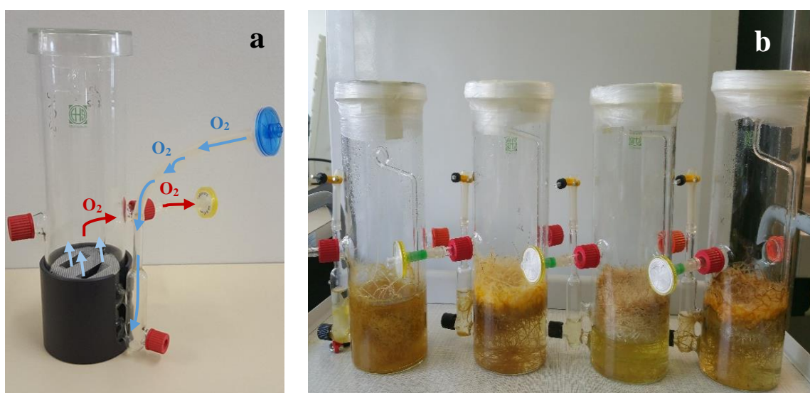
Figure 44: Cultivation of hairy root culture in a Bubble reactor. (A) Bioreactor set-up; (B) Hairy roots obtained after 30 days of growth.
