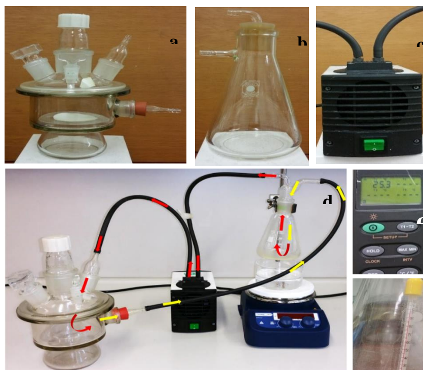
Figure 21: Thermal Releaser; a. exposure part, b. Heating part, c. Air pump, d. Complete thermal releaser device. e. thermometer.
