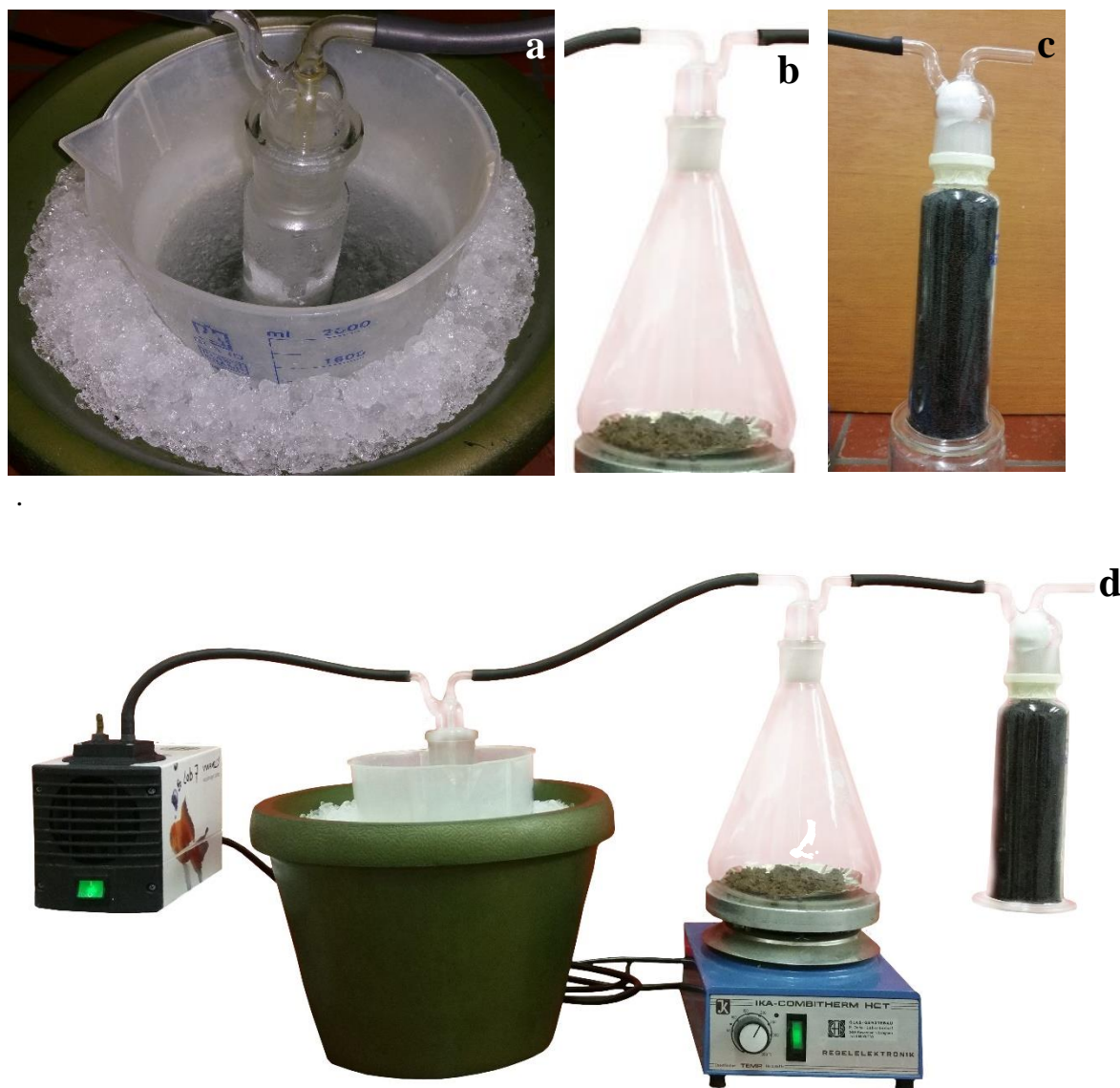
Figure 22: Volatile compound collector; a. Deep freezer -20, b. liquid collector tube, c. Soled (charcoal) collector tube and air filter, d. Complete Volatile collector device.
