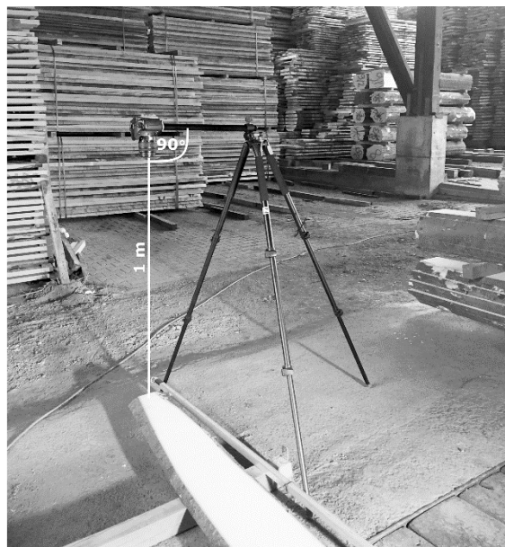
Figure 3.1 Camera arrangement for the image acquisition at the Fehrensen GmbH showing the vertical distance to the board surface of 1 m and the angle to the board surface of 90 ° (created using INKSCAPE version 0.92 and Adobe Photoshop CS3 Extended version 10.0).
