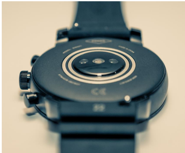
Figure 5. The contact sensor for pulse measurement of a smartwatch
