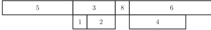
(b) Double-row layout deduced from the schedule above where 8 lies directly opposite 7. Note that department 7 is not drawn because it is larger than department 8 and would overlap with departments 2 and 4.
