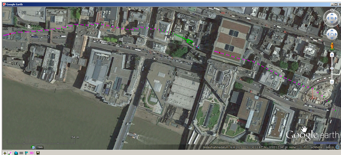
Figure 1.1: Satellite navigation in dense urban areas can be especially difficult, such as in the City of London [Goo15]. The vehicle was driving along the east-west road in the middle of the figure, however the navigation system estimated positions of up to 50 m north of that road, due to tall buildings blocking and reflecting the satellite signals.
