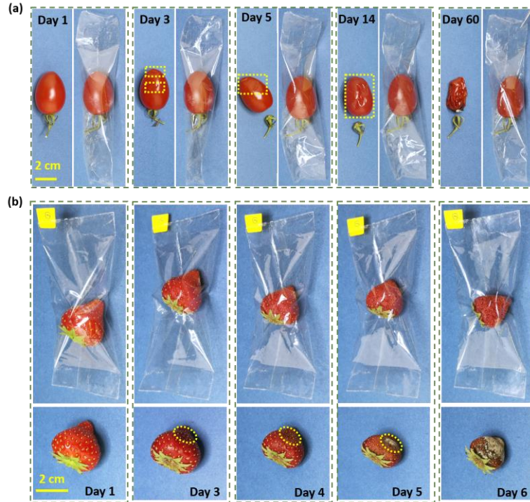
Figure 20 Self-compounded CCi nanocomposite membranes with DS of 0.6 applied as packaging materials for (a) mini-date vine tomatoes and (b) strawberries. The non-packaged and packaged mini-date vine tomatoes were stored in an environment with temperature of 23-25 °C and RH of 70-80 %, while the strawberries were stored in ambient environment with room temperature and RH of 30-40 %. The yellow dashed rectangles in (a) denote the wilted area of non-packaged mini-date vine tomatoes, while the yellow dashed circles in (b) denote the areas with mold spoilage of non-packaged strawberries.
