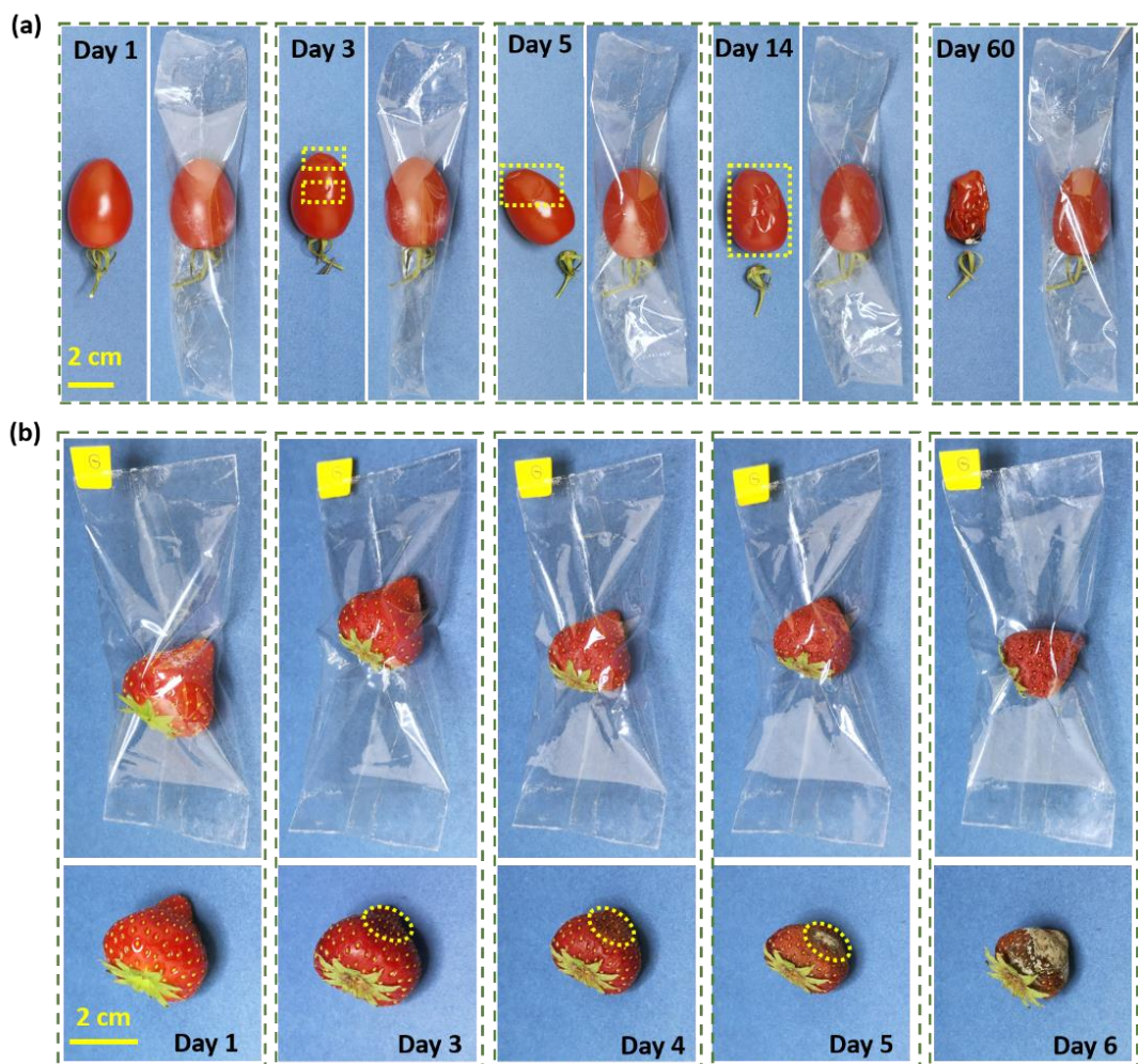
Figure 6. Self-compounded CCI nanocomposite membranes with DS of 0.6 applied as packaging materials for (a) mini-date vine tomatoes and (b) strawberries. The non-packaged and packaged mini-date vine tomatoes were stored in an environment with temperature of 23-25 °C and RH of 70-80 %, while the strawberries were stored in ambient environment with room temperature and RH of 30-40 %. The yellow dashed rectangles in (a) denote the wilted area of non-packaged mini-date vine tomatoes, while the yellow dashed circles in (b) denote the areas with mold spoilage of non-packaged strawberries.
