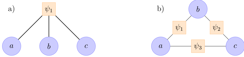
Figure 3.2: Example of a factor graph with three variables a, b, c , denoted by circles and factor nodes denoted by squares. In the factor graph a) only one factor \Psi_1 is used. In the factor graph b) three factors \Psi_1, \Psi_2, \Psi_3 are used. The induced network for both is a clique over a, b, c according to figure B.1 a). The shaded boxes \Psi_1, \dots, \Psi_3 are factor nodes. The set of all distributions p(a, b, c) over the three variables a, b, c can be factorized as p(a, b, c) = \Psi_1(a, b, c) for graph a) and p(a, b, c) = \Psi_1(a, b)\Psi_2(b, c)\Psi_3(a, c) for graph b).
