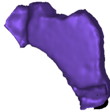
Figure 7.3: A 3D mesh of a HDD magnet acquired from a point cloud. The process starts with component segmentation module that segments the magnet on a 2D plane. Later, the acquired point is used to project the found 2D pixels on the 3D point cloud obtained by the stereo camera. Lastly, using Voxblox [Ole+17], the point cloud is processed into the 3D mesh.
