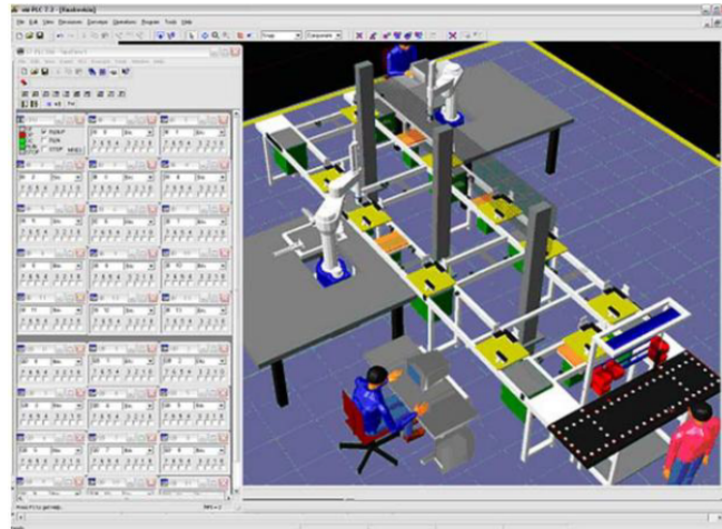
Figure 2.3: Hybrid system for LCD screen disassembly, where humans and automation systems or robots cooperate to achieve the goal of disassembly [KKS09].
