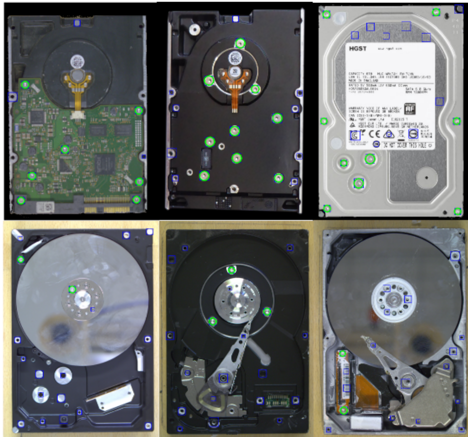
Figure 5.15: Sample outputs of the pipeline. Blue rectangles show the candidates generated by Hough Transform and the green circles refer to the true positives predicted by the ensemble model. The proposed scheme is robust to different backgrounds and to different illumination. In all of the images above, the screws were detected correctly [YW19].
