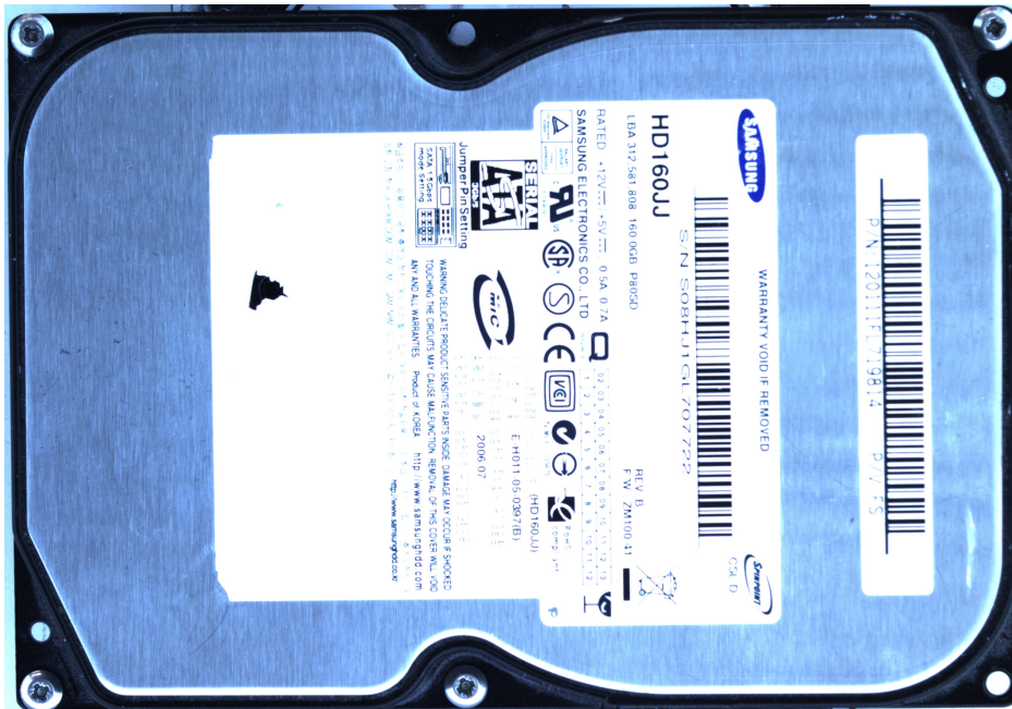
Figure 2.6: A 3.5" computer hard drive with four Phillips-1 screws on its lid.
