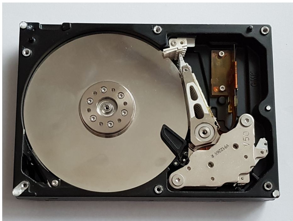
Figure 5.1: Sample hard drive without its lid.
