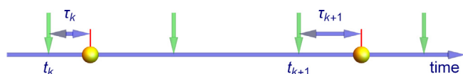
Fig. 3. TTTR counting scheme: single-photon detection events are timed on two different time scales. On a pico- to nanosecond time-scale, the so-called micro-time ( \tau_k ) records the detection time of each photon k (yellow balls) with respect to the last preceding laser pulse (green arrows). If one histograms these micro-times, one obtains the TCSPC fluorescence decay histogram, the bin width of which is determined by the discrete temporal resolution of the micro-times. On a time scale slower than the laser pulse repetition period, absolute arrival times of photons are recorded with a temporal resolution of one laser period (macro-time t_k ). From both time tags, the absolute detection time with an overall temporal resolution of picoseconds can be reconstructed. (For interpretation of the references to colour in this figure caption, the reader is referred to the web version of this article.)
