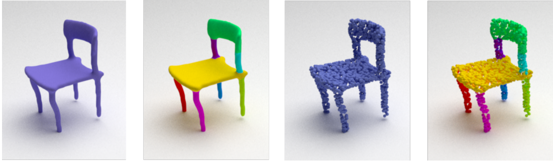
Figure 3.1: Different 3D modalities and respective segmentations. From left to right: Original mesh, segmented mesh, original point cloud, segmented point cloud.
