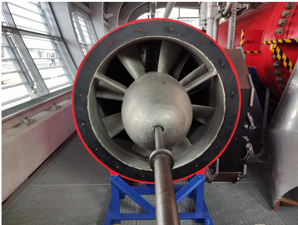
Figure 3.4: Propeller and shaft of the Prandtl wind-tunnel
