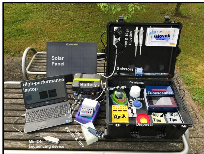
Figure 2. Mobile suitcase lab for the use of Oxford Nanopore sequencing technology at point-of-need (58).
