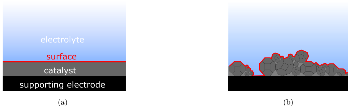
Figure 2.8.: (a) An ideal surface of a catalyst on top of a supporting electrode e.g. a glassy carbon electrode, also called geometric surface as it is only taking into account to macroscopic surface area (b) the electrochemical surface area (ECSA) considering the electrode surface morphology e.g. different particles forming the electrode surface and thereby the interface to the electrolyte.
