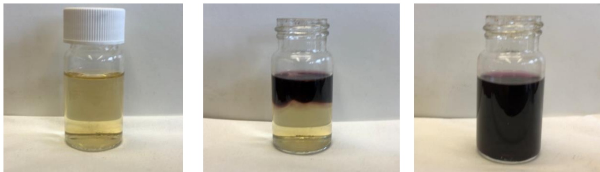
Figure 28. Gradual conversion (left to right) of complex 1 in acetone at room temperature to the corresponding peroxodicopper(II) complex 2 by diffusion of ambient air.
