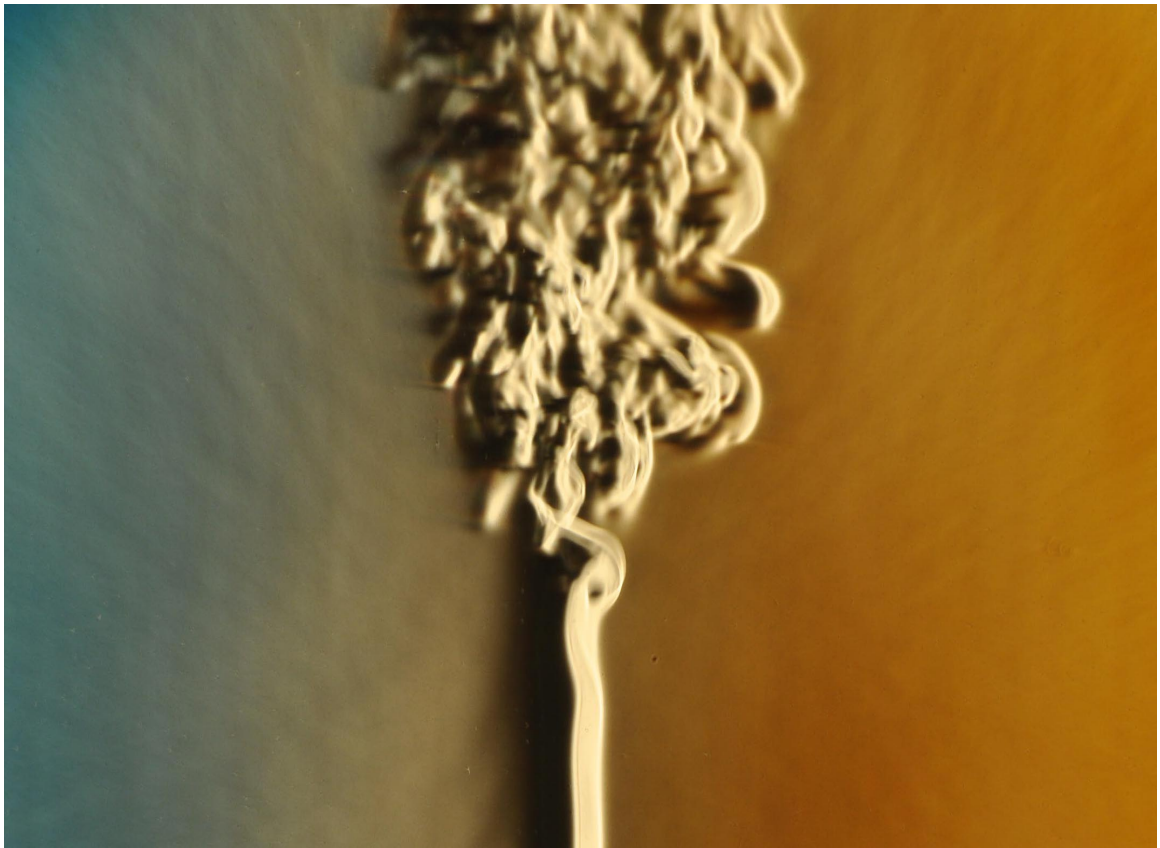
Figure 4.1: The transition from the laminar flow to turbulence flow. Reproduced from [31].
