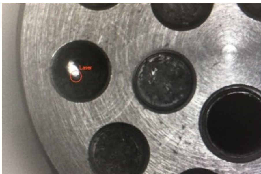
Figure A.6: View into the sample chamber with the camera (May 2019), which is attached to the laser objective. The sample chamber is filled with \text{BrF}_3 and the laser beam is heating the selected sample on the 14-pit sample holder triggering the fluorination. The stronger the reaction the brighter the light emission.
