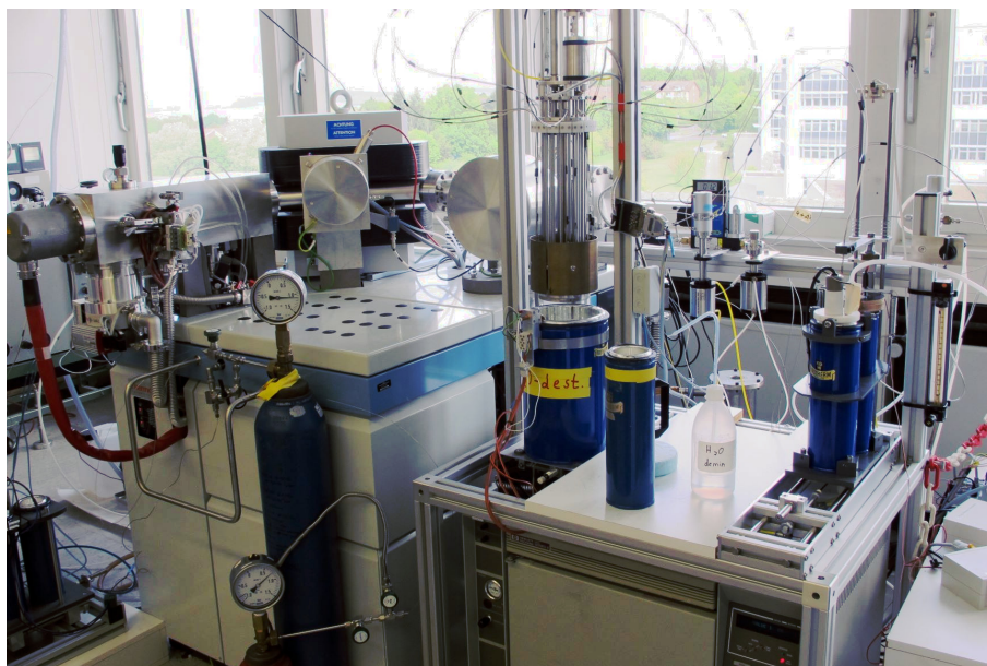
Figure A.2: Image of the Thermo Scientific TM MAT 253 TM IRMS and the automated trap 8 (May 2019).
