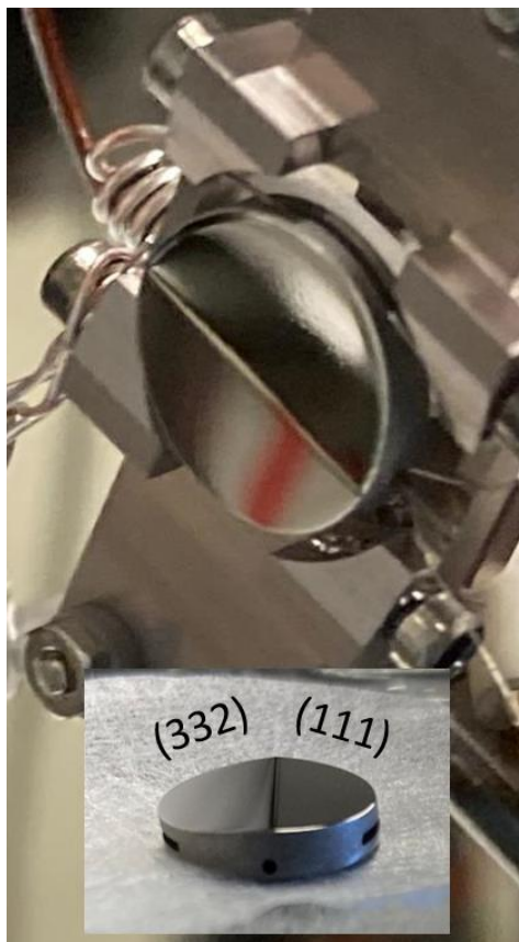
Fig S1: Photograph of the dual facet platinum surface used in this work.
