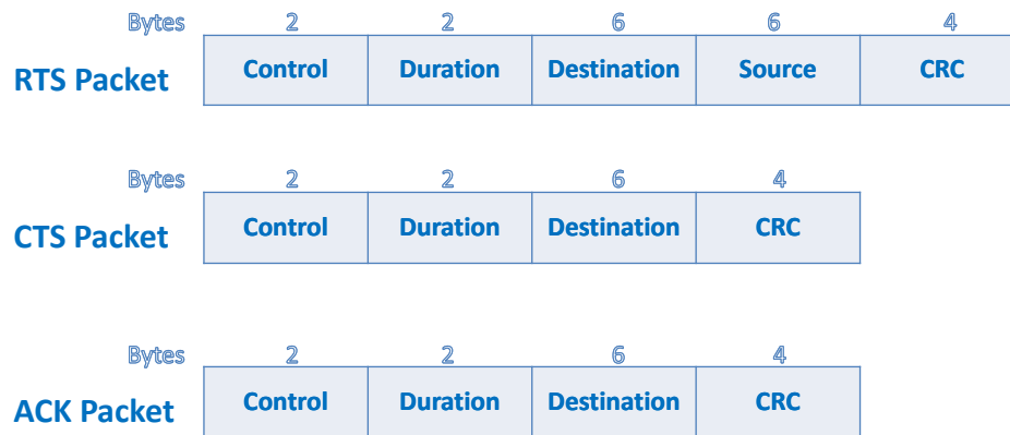
Figure 5.2: IEEE 802.11 MAC layer control packets format.
