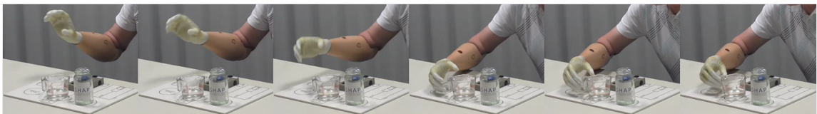
Figure 5.5: Exemplary sequence of Amp2 performing simultaneous wrist flexion and supination followed by a pinch grip to grasp the mug of the SHAP test.
