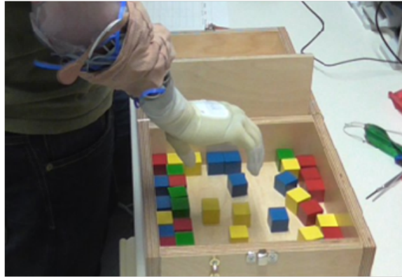
(a) A subject performing the box and blocks test. As many cubes as possible have to be transferred from the one box to the other over the barrier between them.
