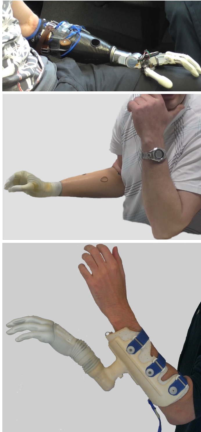
Figure 4.4: Prosthesis mounted on subjects. Upper two panels: one right (Amp1) and one left (Amp2) hand amputee, lowest panel: adapter for able-bodied subjects to wear the prosthesis for the tests. Reused and modified with permission [84] ©2014 IEEE.
