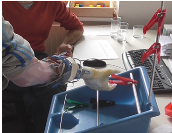
(b) A subject performing the clothes pin test. The task was to relocate the clothes pin from the lower, horizontal bar to the upper, vertical bar.
