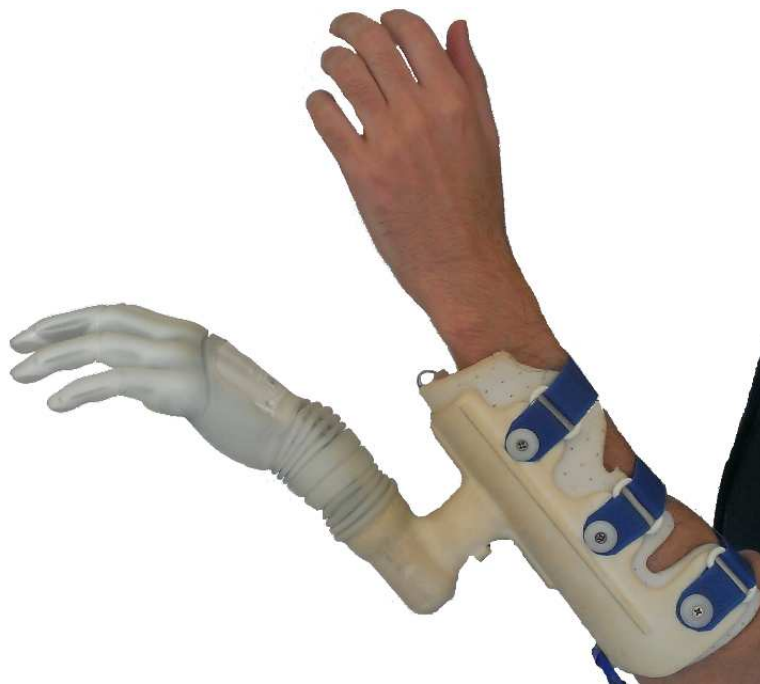
Figure 3.8: The Michelangelo hand prosthesis (Otto Bock HealthCare GmbH, Germany) and special socket for usage with able-bodied subjects. Both stimulation electrode and EMG recording electrodes were placed within the socket. Photo courtesy of Sebastian Amsuess.
