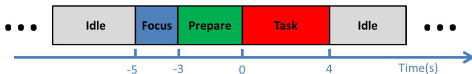
Figure 2.5: Experiment procedure with different motor tasks. Each trial began with an idle phase, followed by a 2-s focus phase and a 3-s preparation phase. In the consequential task phase, the subject was instructed to perform ballistic or repetitive imagination of dorsiflexion.
