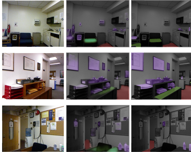
Figure 5.8: Probabilistic segmentations generated using our method on the NYUv2 dataset [186]. Columns (left to right): original image, predictions of P105, and ground truth.
