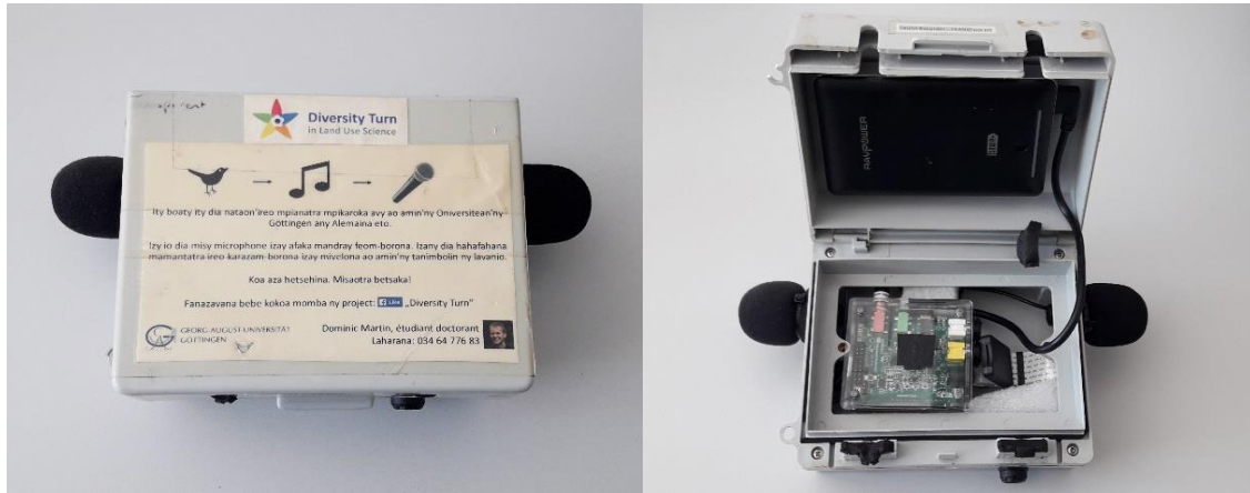
Figure 12.4: Self-built SOLO audio recorders used for sound recordings. a) Closed recorder with two omni-directional microphones including windshield foams and labelling in local Malagasy language to explain research method. b) Opened recorder showing its configuration based on a Raspberry Pi A+ model, Cirrus Logic audio card, PiFace Real Time Clock Module and a standard USB battery pack.
