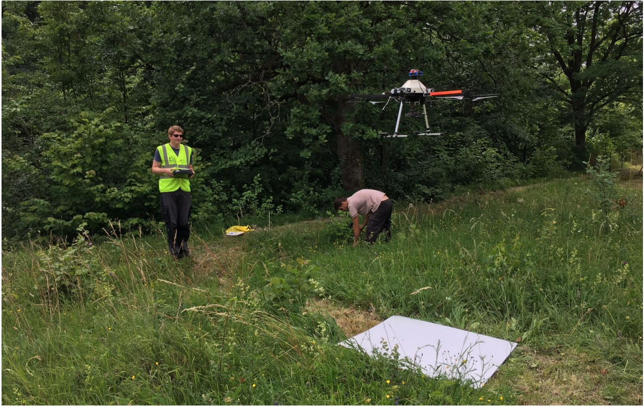
Figure 1. Unmanned aerial vehicle (octocopter) used for the assessment of the flower diversity of calcareous grasslands. © Maxim Bogdanowitsch.
