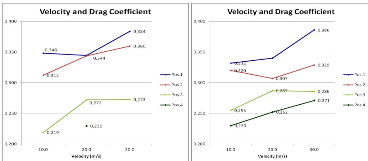
Figures 26 and 27 – Performance curves for  $C_D$  according to test stages performed in 2010 and 2011.
