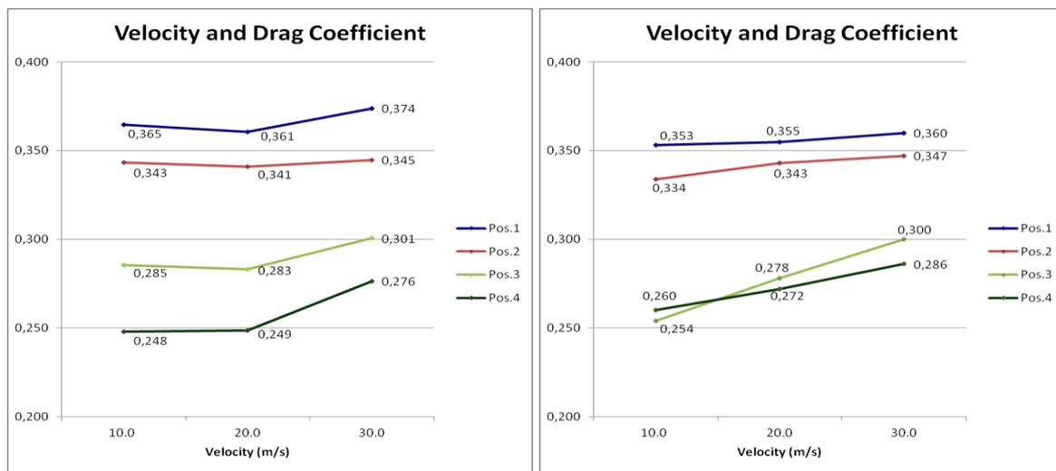
Figures 9 and 10 – Performance curves for  $C_D$  according to test stages performed in 2010 and 2011.
