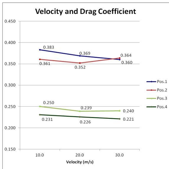
Figures 61 and 62 – Performance curves for **C<sub>D</sub>** according to test stages performed in 2010 and 2011.
