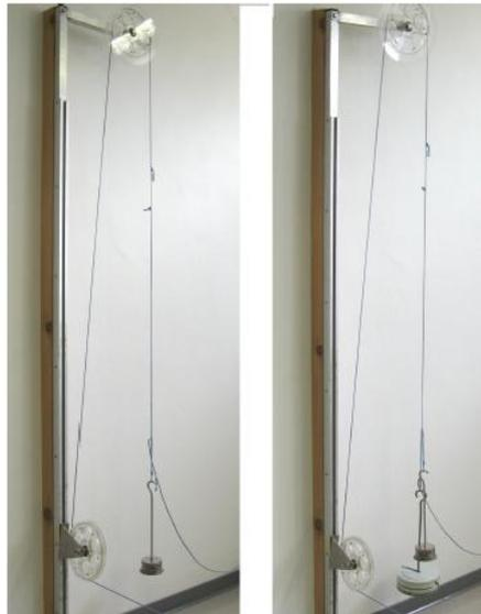
Fig. 15: Pulley System, auxiliary force admission.
