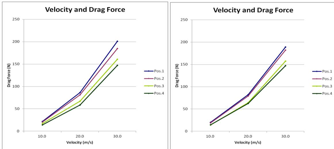
Figures 7 and 8 – Performance curves for  $D$  according to test stages performed in 2010 and 2011.
