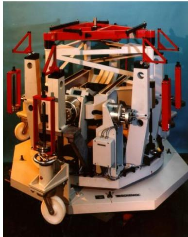
Fig. 22: Six-component (External) Balance (<http://www.tu-harburg.de>).
