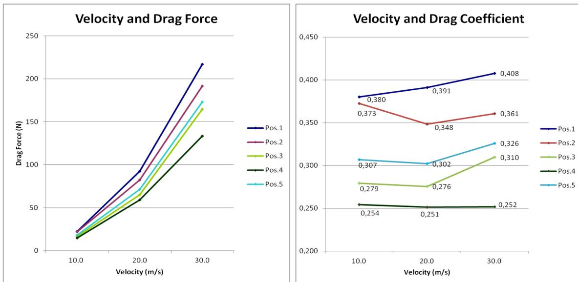
Figures 75 and 76 – Performance curves for **D** and **C<sub>D</sub>** according to test stage performed in 2010.
