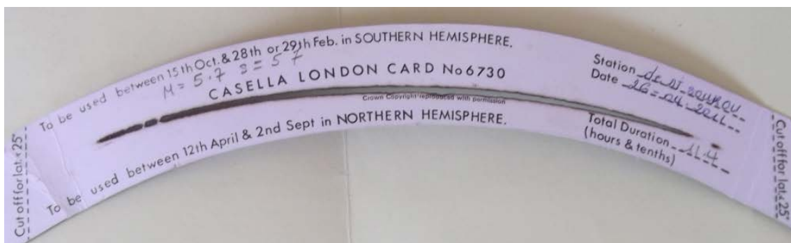
Figure 74: Sunshine recorder card on 2011/04/26 used at Di-Sourou weather station
