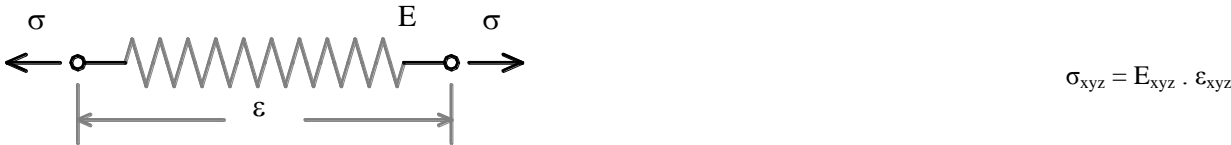
Figure 4. Model with elastic behaviour, \sigma_{xyz} and \epsilon_{xyz} they are, stress and unitary deformations for each one of the main direction, E_{xyz} means the proportionality constant for the corresponding direction, which conventionally represents E or MOE
