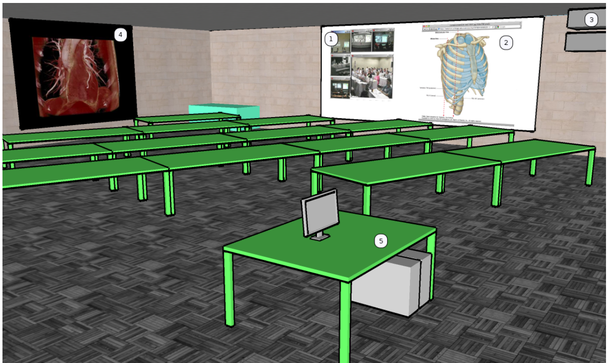
Figure 2.3. The class had two projection screens: The first was served by a single projector and presented video of the remote audience (1) and 2D illustrations (2), the second (4) was served by two projectors (3) and presented the stereoscopic visualization. The technical setup was controlled from a dedicated workplace (5).
