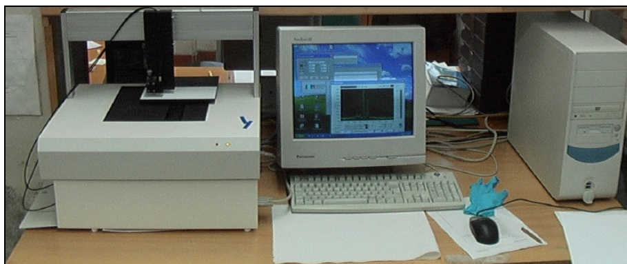
Figure 8: Multi-wavelength TLC-scanner which is a developed UV-Spectrometer with X-Y scanning ability for TLC plates
