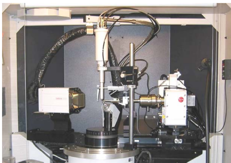
Figure 3-6: BRUKER TXS Mo rotating anode equipped with an APEX II CCD detector and INCOATEC Helios mirror optics as monochromator.
