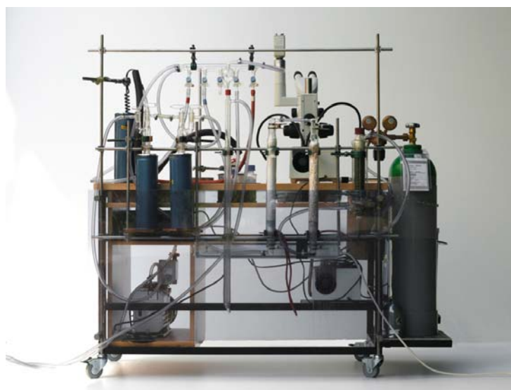
Figure 3-5: Back view of the table for crystal mounting with gas drying system.
