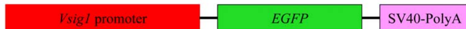
Figure 3.43 Schematic representation of the transgenic construct. The Vsig1-EGFP construct contains the coding region of the EGFP gene (cDNA) under the control of a 4.8-kb Vsig1 promoter and SV40 polyadenylation signal (SV40).
