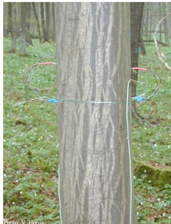
Figure 5. Sensor insertion into the trunk of beech trees. Sensors were placed at 1.3 m height above the trunk base and 10-15 cm apart from each other (left) (upper (red): heated, lower (blue): unheated sensor on opposite, northern and southern directions (right).
