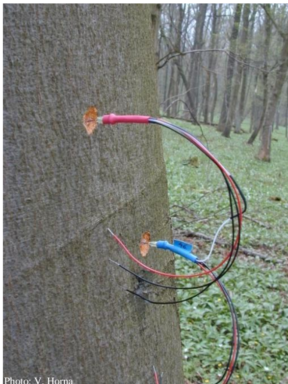
Figure 5. Sensor insertion into the trunk of beech trees. Sensors were placed at 1.3 m height above the trunk base and 10-15 cm apart from each other (left) (upper (red): heated, lower (blue): unheated sensor on opposite, northern and southern directions (right).
