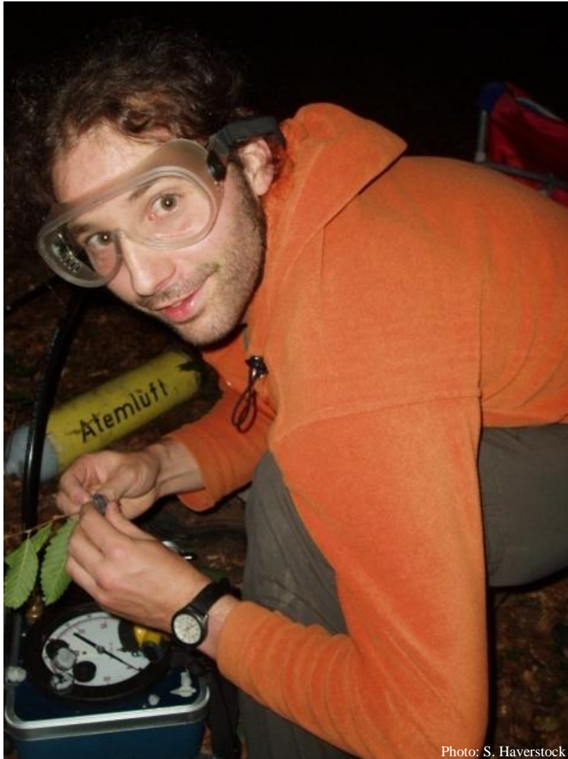
Figure 10. Measurement of predawn and noon leaf water potentials with the Scholander pressure chamber. Here, a hornbeam twig is placed into the rubber sealing before insertion into the pressure chamber to start the predawn leaf water potential measurement.
