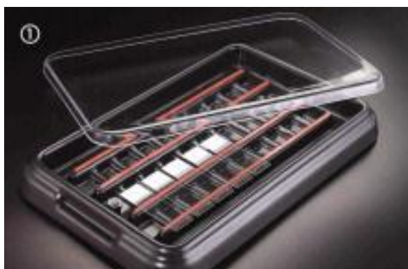
Figure 10: Incubation chamber for the microarray chip (Rotilabo ® -Färbekammern, CARL ROTH GmbH, Karlsruhe).
