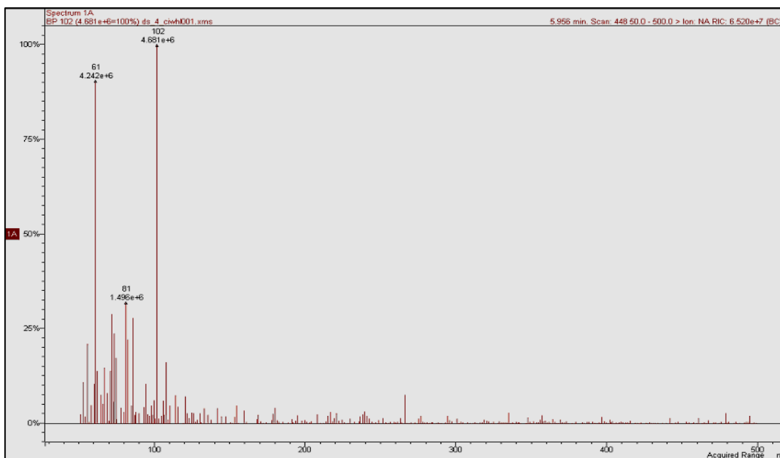
Figure 3.11: Mass spectrum of m/z 210 \text{KNO}_3 in ESI negative mode.
