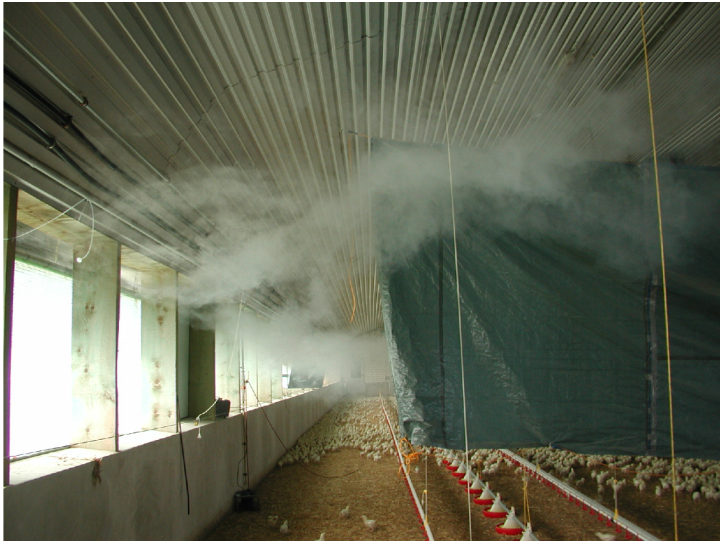
Fig. 3- 5: Smoke test displays air mixing within the broiler house and air mixing sub-section
