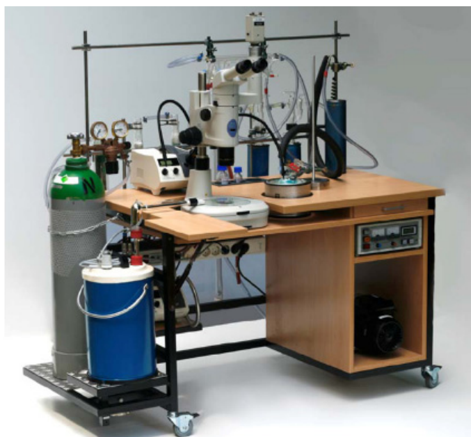
Figure 8-1: Mounting table with the X-TEMP2 cooling device. [214]
