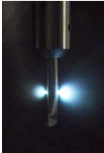
Figure 3.3: High harmonic generation by focussing the 800 nm fundamental light pulses into argon gas escaping from a metal capillary, whereby plasma fluorescence can be observed, resulting from the hole burning process.
