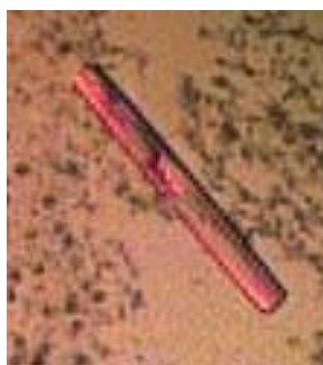
Figure II-21. A crystal of the AE2 form. The long sides of the needle were always slightly curved and the crystals would only grow weeks after microcrystals or precipitate had developed in the drops.
