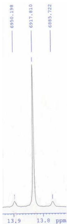
Figure 8. Section of the ^1\text{H} NMR spectrum (500 MHz, \text{C}_6\text{D}_6 ) of 15 showing the Sn–H proton resonance flanked by tin satellites.
