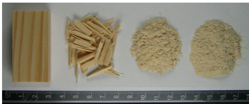
Fig. 1 A. grandis (left to right) wood block [50 (longitudinal) x 20 (tangential) x 15 (radial) mm], wood shaving after chipping, wood powder after grinding and wood powder after Soxhlet extraction
