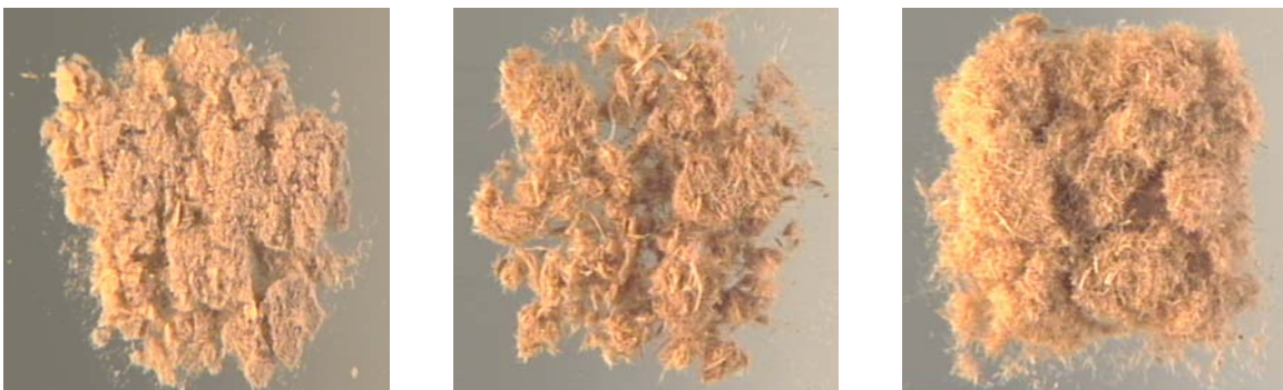
Figure 16: Dried UF-recycling fibers after the thermo-hydrolytic process (left part of the picture), after gluing with MUF-resin (middle of the picture), and after refining in the Pallmann-mill PXL 18.
