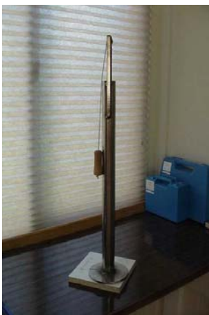
Figure 14: Determination of impact strength according to UNE-standard 11019/6
