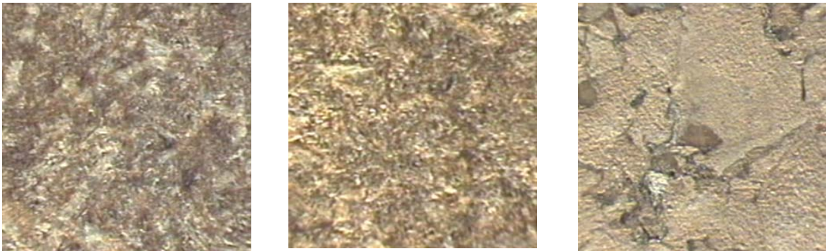
Figure 42: Images from uncoated TF-bonded medium density fiberboards (MDF), made using raw materials in the surface layers (fresh fibers (left), recycled fibers (middle) and cork particles (right)). The boards were stored under 20°C / 65% relative humidity.
