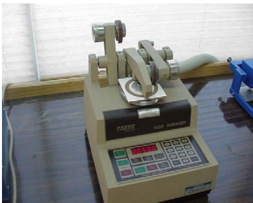
Figure 15: Determination of abrasion strength with a Taber abrasion instrument according to EN-standard 438-2, article 6
