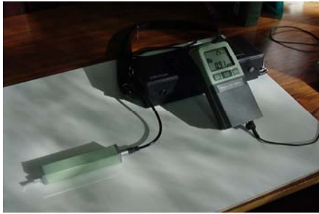
Figure 10: Roughness measurement of a particleboard coated with nitrocellulosic paint.
