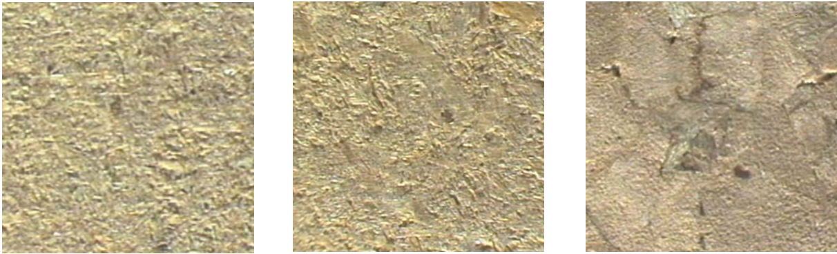
Figure 39: Images from uncoated MUF-bonded medium density fiberboards (MDF), made using different raw materials in the surface layers (fresh fibers (left), recycled fibers (middle) and cork particles (right)). The MDF were stored under 20°C / 65% relative humidity.
