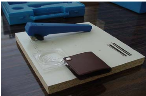
Figure 12: Determination of adherence strength according to UNE-standard 48032
