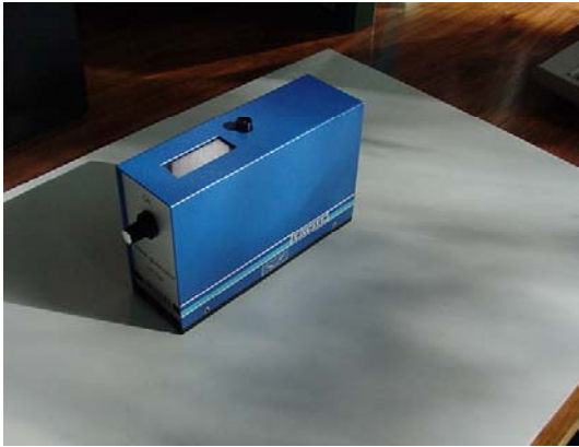
Figure 13: Determination of speculate brightness according to UNE-standard 48026
